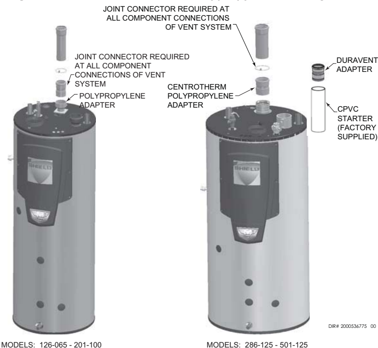
Figure 2-9 Near Water Heater Polypropylene Venting
